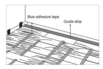
• Use blue adhesive tape every five or six rows to ensure planks remain firmly in place.
